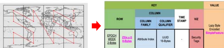
Figure 3. GeoMesa's data indexing scheme (Left) and the real structure of index in Accumulo (Right). The red line shown in left panel is known as a Z-curve. The Z3 encoding (x,y,t) shown in right panel is used to efficiently answer queries of features with point geometry with both spatial and temporal components.
